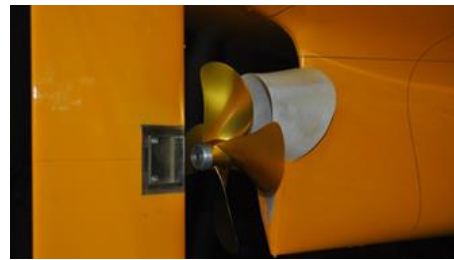
Figure 3: Neighbor Duct for 82kBC in model test
