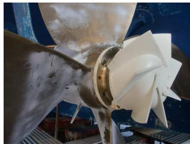
Fig.1 ECO-Cap attached to the actual ship
